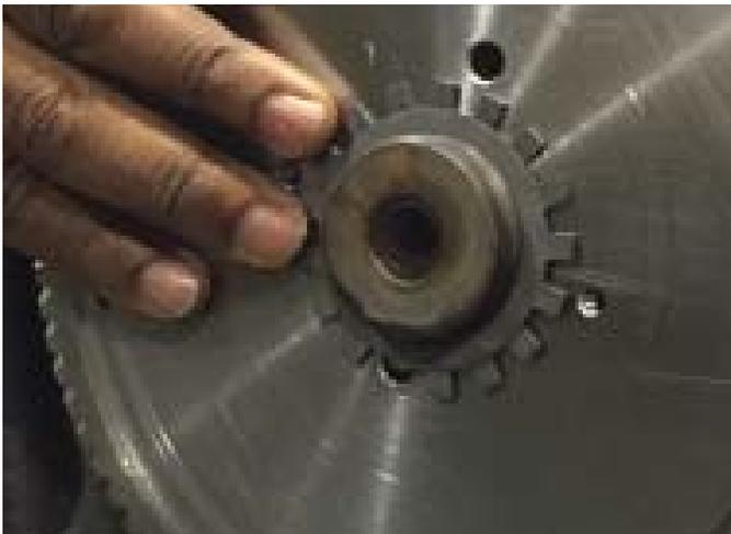
Figure 9-5 Tab on Washer Must Seat Into Slot on Timing Gear
