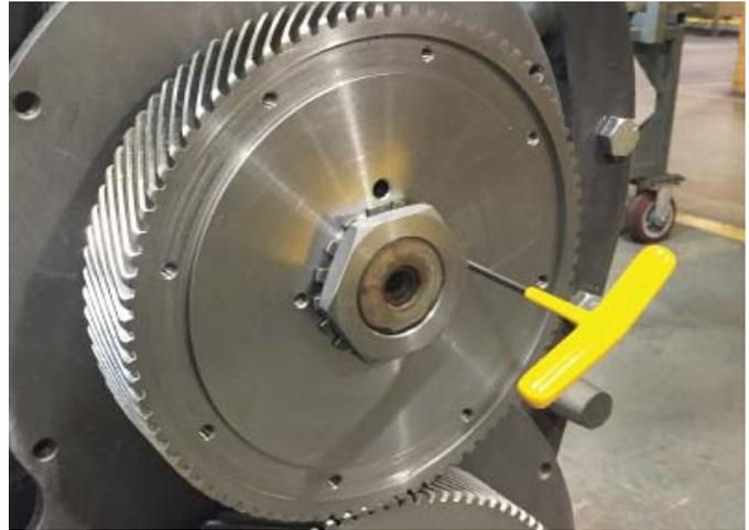
Figure 9-11 Proper Method for Setting Rotor End Clearance
