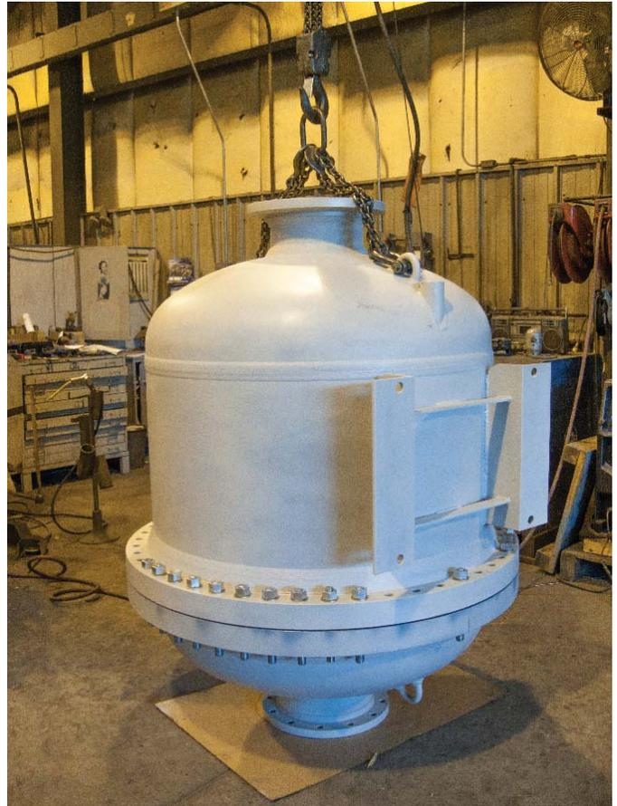
Figure 9-15 Position Meter Housing and Replace all Bolts To Proper Torque
