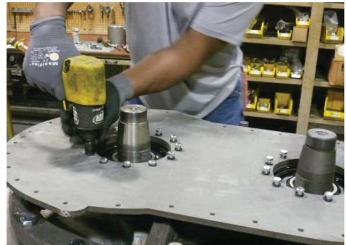
Figure 10-10 Replace and Secure Mounting Plate With Screws and Washers
