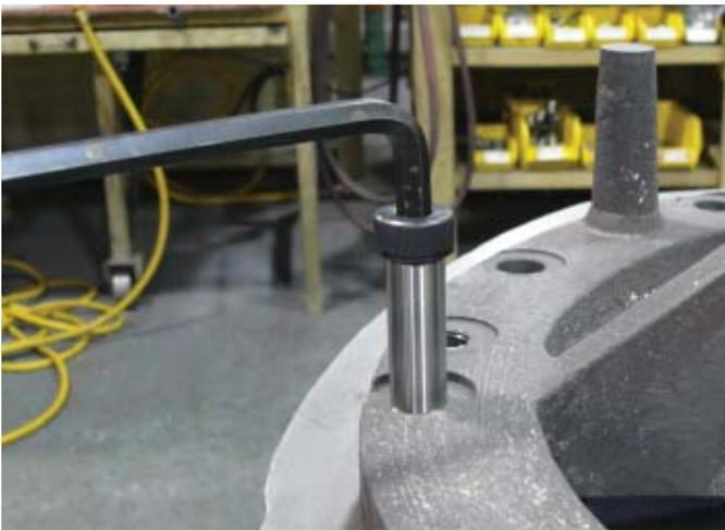
Figure 9-2 Align Two Dowel Screws with Their Corresponding Holes
