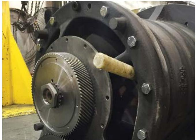
Figure 9-1 Proper Method for Blocking Rotors
