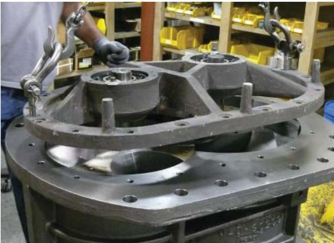
Figure 9-8 Position and Lower Rear End Plate in Place
