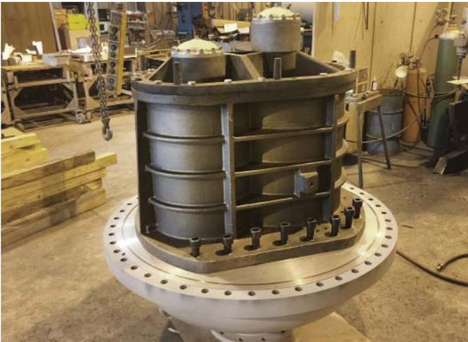
Figure 9-14 Connect Measuring Unit to End Cover and Secure all Nuts to Their Proper Torque
