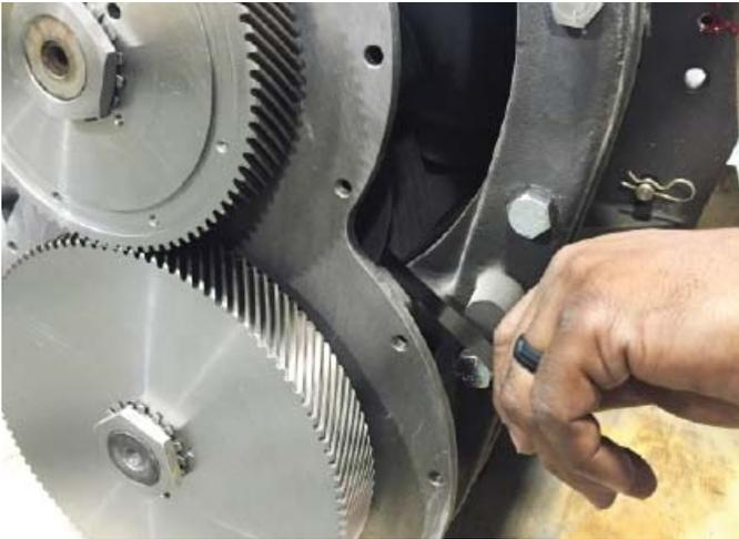
Figure 9-12 Proper Method For Timing Gear Adjustment
