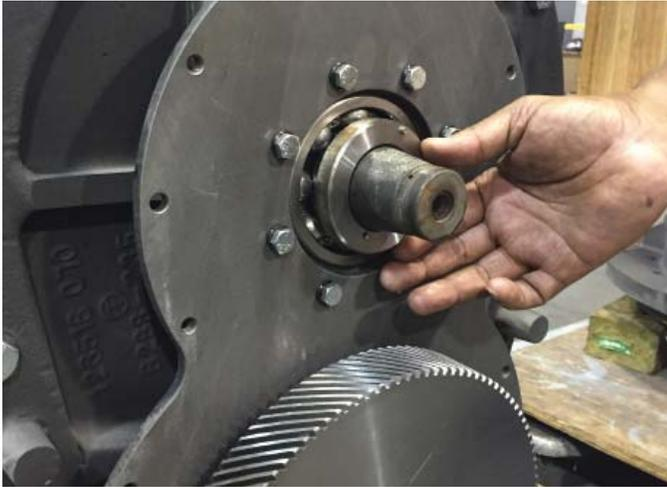
Figure 9-4 Install Rotor Spacer and Slide Timing Gears onto Proper Shaft Before Replacing Loackwashers
