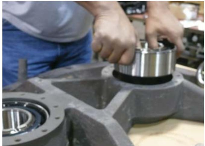
Figure 9-3 Install Ball Bearings into Bearing Bore Provided in End Plate
