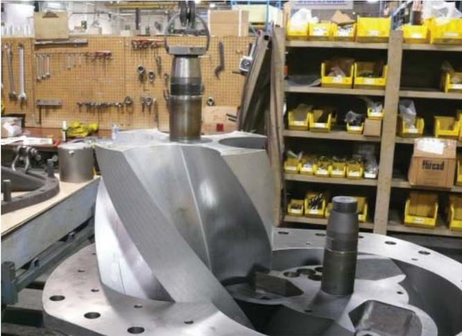
Figure 9-7 Position the Rotors and Lower into the Appropriate Cavity
