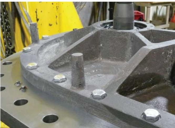
Figure 9-9 Secure End Plate to Measuring Unit Body
