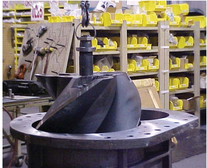
Figure 2: Install 4 Tooth Rotor
